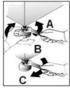
Level the machine using the front feet Turn the nut clockwise to unlock the screw adjuster.
