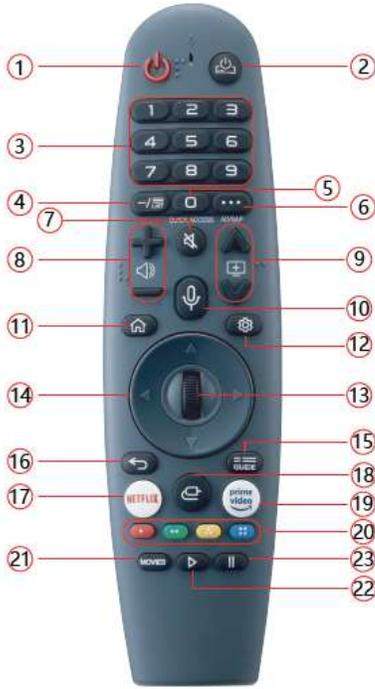
1. **POWER:** To switch the device on or standby
