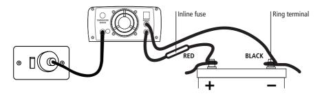
If the charger is used in a Permanent/Hard Wired application and the vehicle will not be used for some time, it is best to leave the charger connected to mains power (turned 'On') so that it can maintain the battery fully charged.
