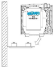
Installation on Vertical bulkhead
