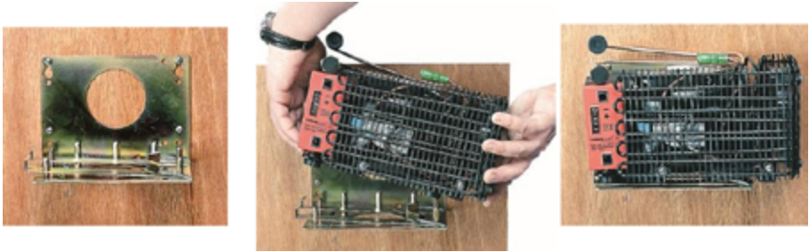
Figure 5: Detail of compressor unit - bracket attachment
