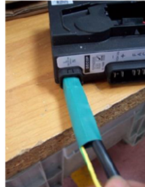
Figure 11: Detail of double insulated connection
