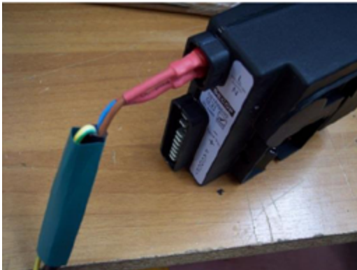
Figure 11: Detail of double insulated connection
