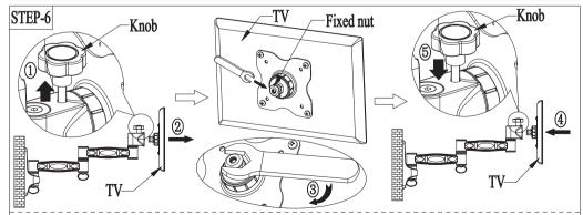
Please fasten the fixed nut as below procedure if the tilt angle cannot be fixed properly. Loosen the knob at first, then remove the TV together with the TV plate from the wall plate, Firmly tighten the fixed nut with a spanner in the clockwise direction. Insert the TV back to the wall plate, Tighten the knob to the TV plate tightly at last.
