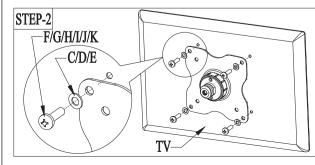
Install TV plate on the TV back. Select four suitable bolts from the parts bag and screw them into the bolt-holes in the back of the TV. The TV plate mounted on the TV back should be mounted symmetrically and evenly.
