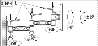
Adjust the position and angle of the flat panel TV for convenient viewing. Using the inner hexagon spanner S=4 (L) to loosen the bolt before adjusting the view angle, and firmly tighten the bolt after adjustment. While adjusting, please take care of your hand to avoid clipping.
