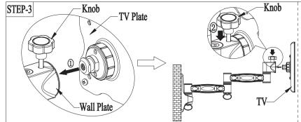
Lift the TV by two person, Insert the TV together with the TV plate into the wall plate, then tighten the knob firmly.
