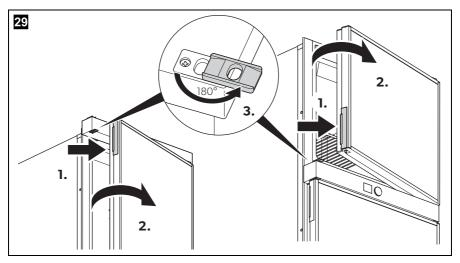
➤ Rotate the locking catch 180° to latch the doors slightly opened (fig. 29).
