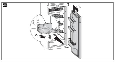
➤ Remove the refrigerator door by lifting it up until it clears the lower pin (1. in fig. 44).
