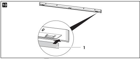
A sealing strip (fig. 10) is applied to the lower surface of the bottom trim piece.
