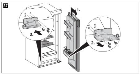
➤ Remove the refrigerator door by lifting it up until it clears the lower pin (1. in fig. 37).
