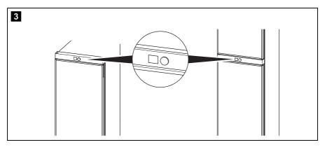
The refrigerator has a display and a control knob above the refrigerator door (fig. 3).
