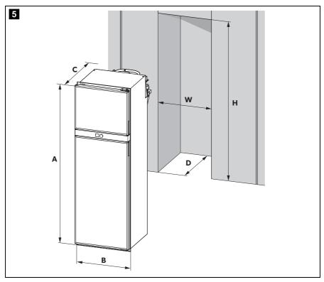
The refrigerator must be installed in a recess so that it stands secure when the vehicle is in motion. Note the following dimensions (fig. 4 and fig. 5):
