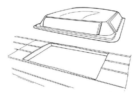
Step 2:- Test fit hatch into cut out area and adjust to suit.
