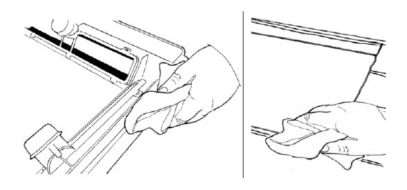
**Step 5:-** Apply a continuous bead of Non Acetic silicone a minimum of 6mm wide to the centre of the foam tape all the way around the hatch. **Do not over apply.**
